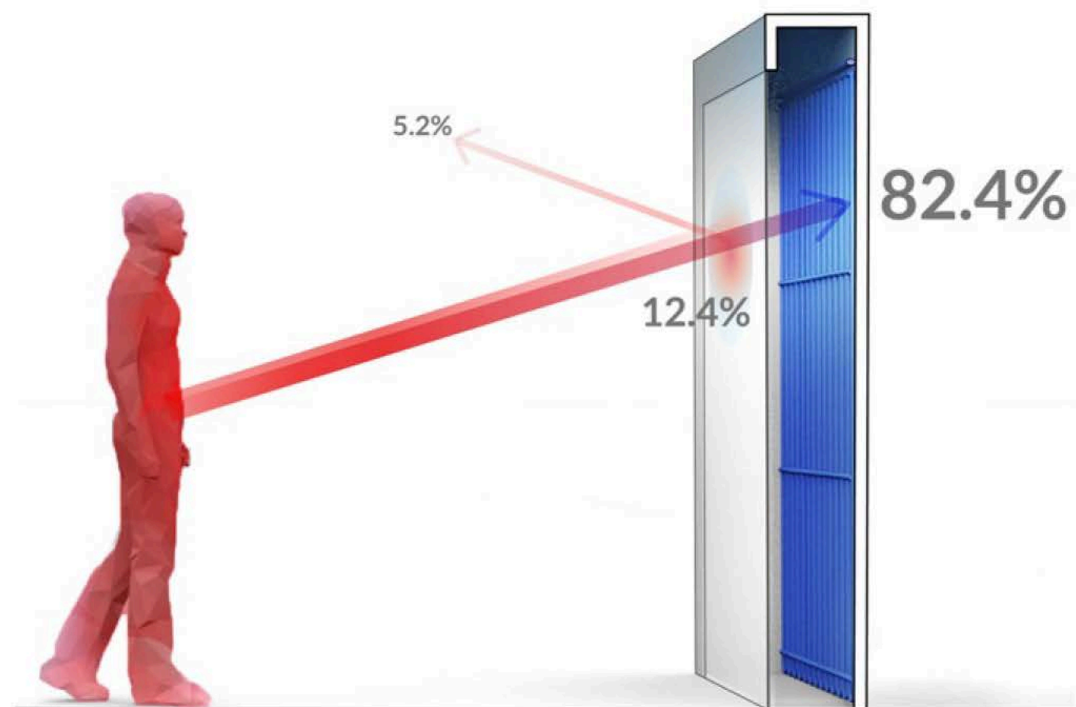
Fig. 1. Schematic of a Cold Tube radiant cooling panel (Upper) and radiant heat transfer through the IR-transparent membrane (Lower).
